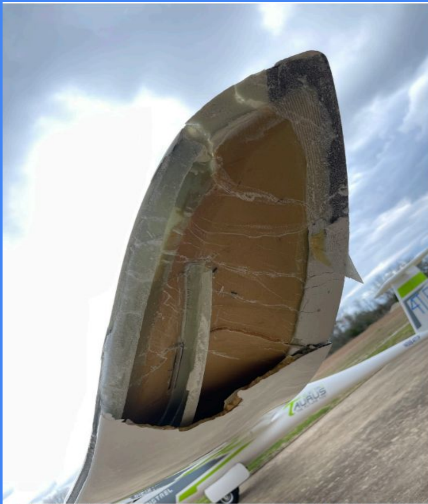
- Pipistrel Glider with Damaged Left Wing (Courtesy of FAA)
